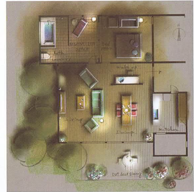
17 Use a computer to create the lighting effects. I use Adobe Photoshop®. Select "Layers" from the "Toolbar." The screen will momentarily go black. Set the "Opacity" level to 50%, select the "Eraser" tool from the "Toolbox," and create the lighting effects.
