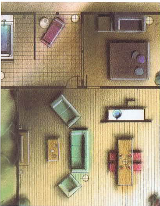
15 Use a finger to smudge the pastel shadows. Use a white colored pencil to add highlights to the sides of surfaces opposite those shaded.
